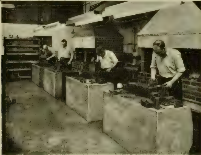
Fig. 1. Hand-forging of surgical instruments
